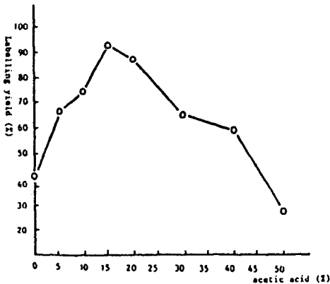
Fig. 2 Labelling yields of reaction in solvent of different acetic acid/ethanol ratio. The percentage of ice acetic acid: 0%, 5%, 10%, 20%, 30%, 40%.
